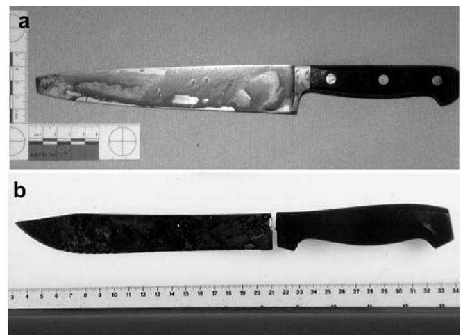
Fig. 2a Knife used in case 3 with anatomically shaped handle and blade wider than the grip. Blade tip broken during attack. b Knife used in case 4 with anatomically shaped handle, so-called clip point blade. Total blade broken off during offence
